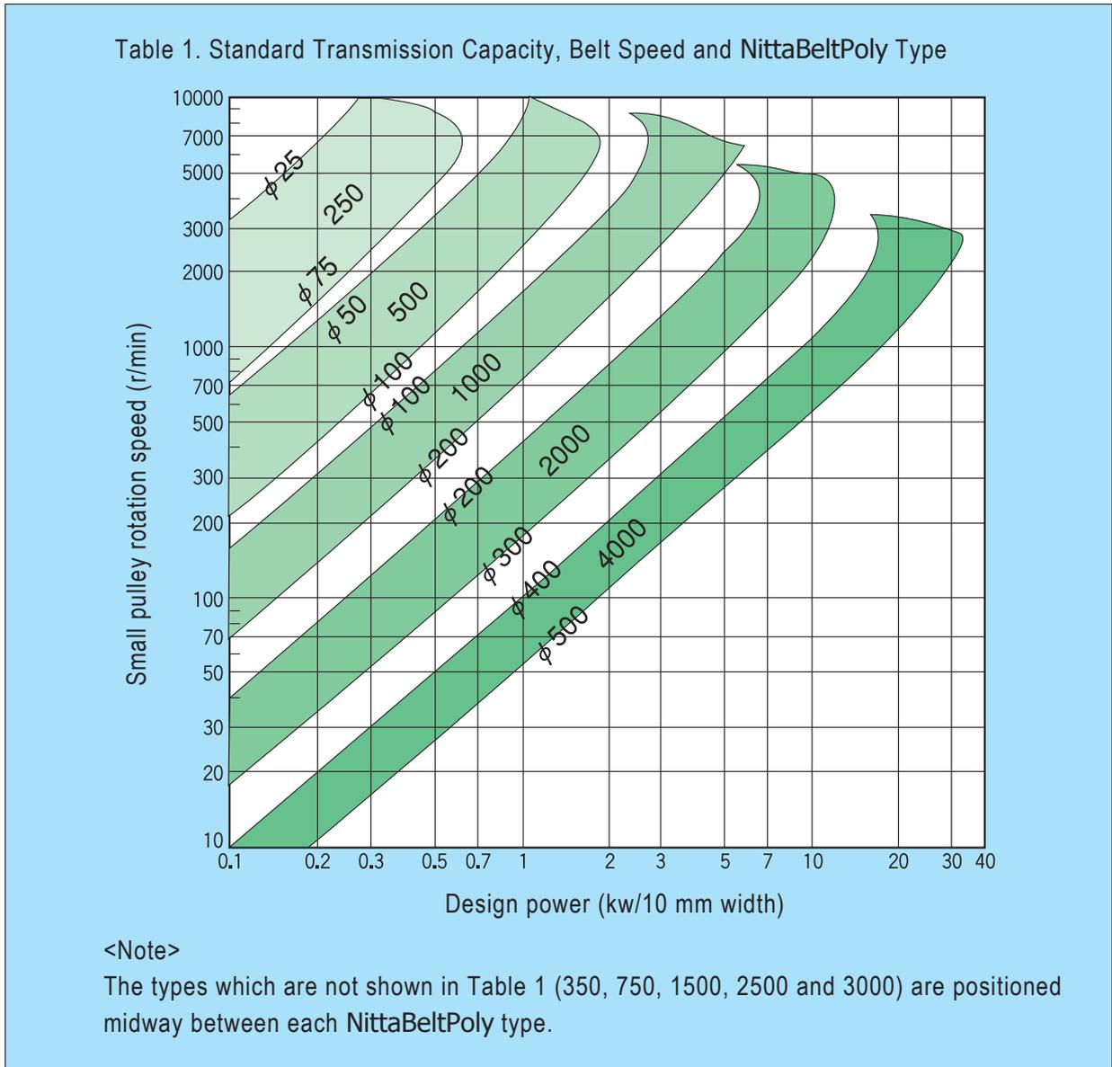
(2) Calculate the belt speed (V) by using the pulley diameter and rotation speed.
