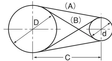
The length of NittaBeltPoly is determined according to the pitch length (Lc). Convert “Li” obtained above into “Lc” .
